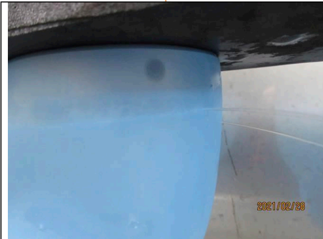
(65) water leakage test(2pc leak)
