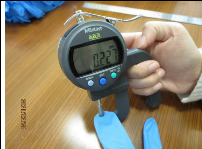
(61)thickness check on fingertip
