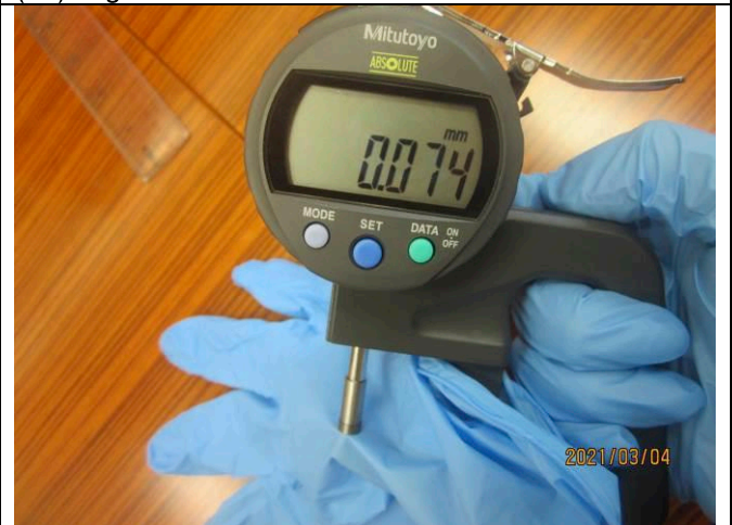
(97)thickness check on palm
