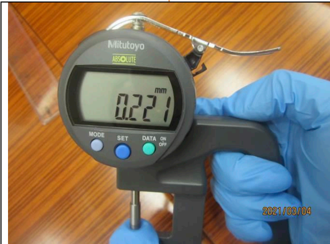
(98) thickness check of finer
