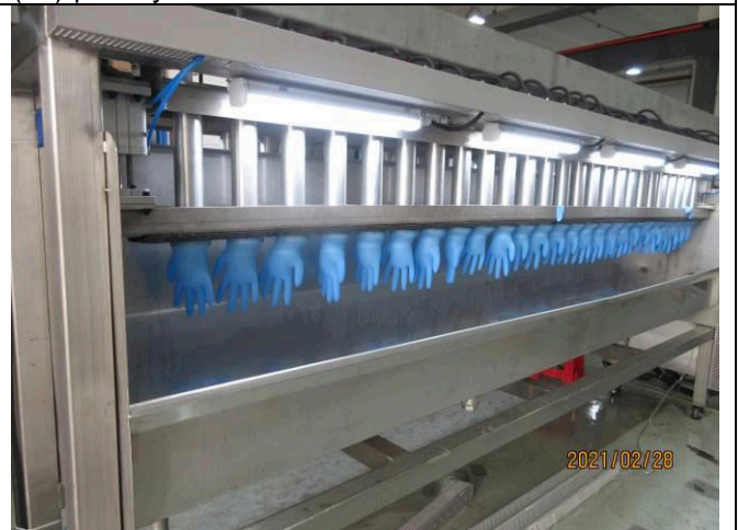
(64)water leakage test
