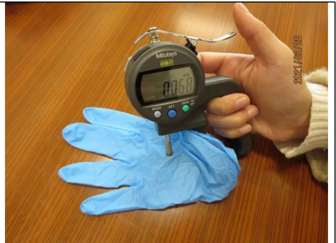
(60)thickness check on palm
