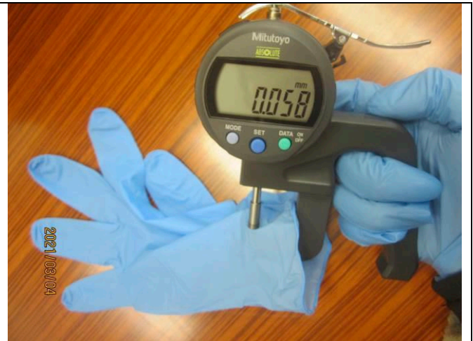
(51)thickness test on cuff
