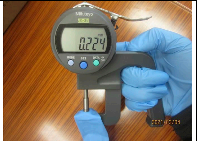
(53)thickness test on finger
